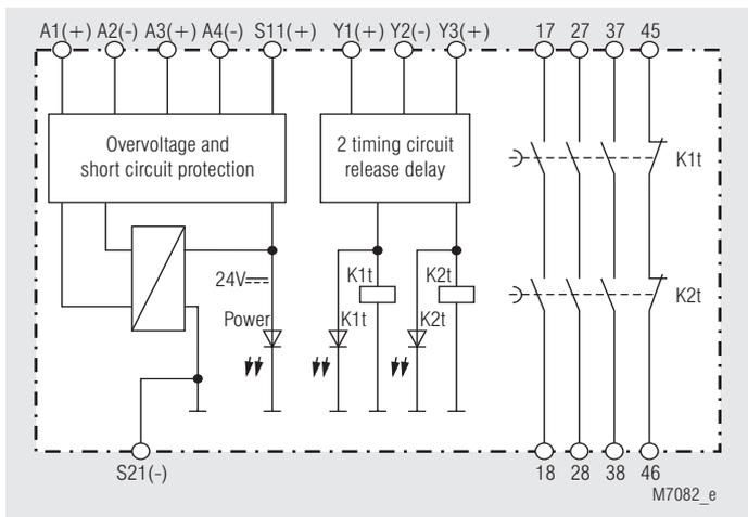
Block diagram for units with 2 timing circuits.
